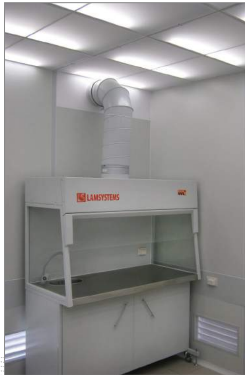
A clean zone for control of special cleanliness materials Cleanliness class 5 ISO 14644-1 or class A GMP Assembly overall dimensions (LxWxH, mm): 7480x3815x3190
