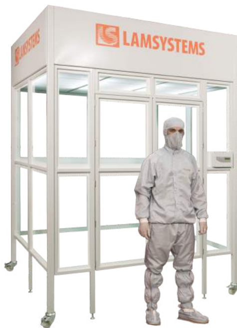
A clean zone for pharmaceutical laboratory Cleanliness class 5 ISO 14644-1 or class A GMP Assembly overall dimensions (LxWxH, mm) 1905x1605x2580
