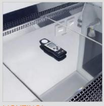
LIGHTING\* corresponds to the requirements of safe operation in the work zone. The illumination of the work zone surface is 2000 lx while the recommended one is 750 lx.
