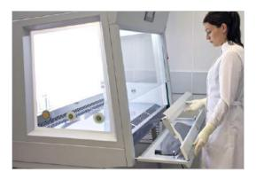
The cabinet has a pullout UV unit which is placed at the bottom of the cabinet (outside contamination zone).
