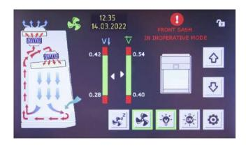
LAMINAR FLOW FAILURE! FRONT SASH IN INOPERATIVE MODE! LOW INFLOW VELOCITY! HIGH INFLOW VELOCITY! LOW DOWNFLOW VELOCITY! HIGH DOWNFLOW VELOCITY! NO CONNECTION TO SYSTEM BOARD
