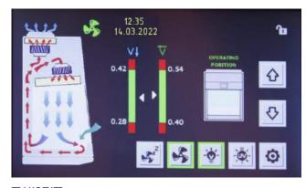
The cabinet is featured with a microprocessor control system that immediately informs an operator on the reduction of the level of the cabinet protection via alarm messages displayed on the touchscreen and via an audible and visible alert.
