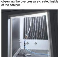
AIRFLOW VISUALIZATION demonstrates the accuracy of airflow distribution and direction.
