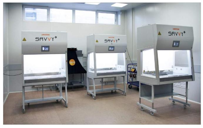
The acceptance testing site is designed as a Class 7 clean room and is fitted with qualified equipment for testing each item released. The acceptance test of SAVVY SL consists of 23 obligatory checks the results of which are registered in a corresponding report. A copy of the acceptance test report can be enclosed to the Manual as per customer's request.
