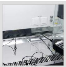
VIBRATION\* The root-mean-square displacement caused by vibration at the tabletop centre of the operating cabinet does not exceed 0.005 mm.
