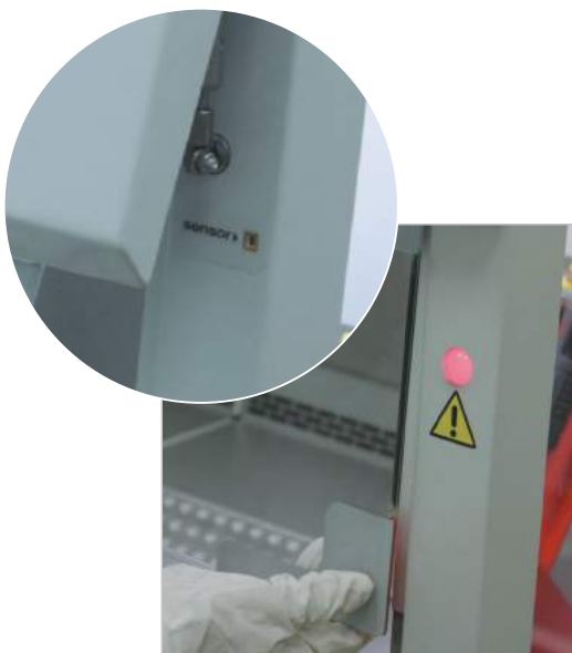
Fig. 1 and 2: Position of the moving and removable parts that effect the protective capacity of the cabinet is controlled by high-precision optical sensors.
