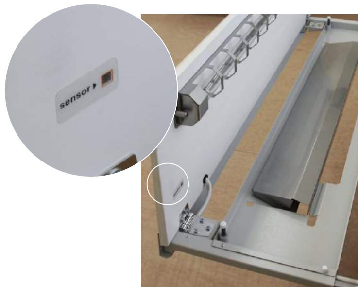
Fig. 1 and 2: Position of the moving and removable parts that effect the protective capacity of the cabinet is controlled by high-precision optical sensors.
