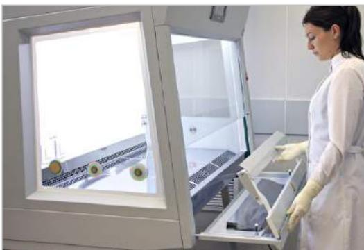
The cabinet has a pullout UV unit which is placed at the bottom of the cabinet (outside contamination zone).
