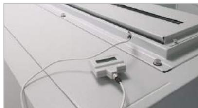
Measuring the Temperature of the Air Outflow
