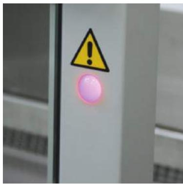
Alarms are automatically activated in case the airflow parameters deviate from the preset values.
