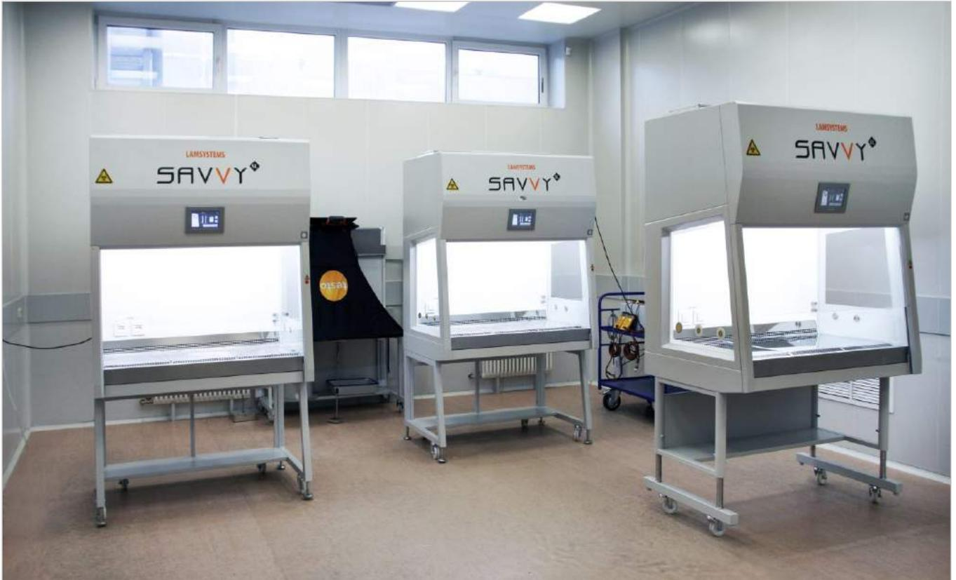
The acceptance testing site is designed as a Class 7 clean room and is fitted with qualified equipment for testing each item released. The acceptance test of SAVVY SL consists of 23 obligatory checks the results of which are registered in a corresponding report. A copy of the acceptance test report can be enclosed to the Manual as per customer's request.
